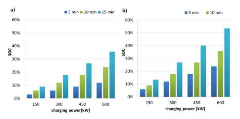
*Fig. 6. Percentage of energy stored in the battery during charging of the battery with an energy capacity of a)* 300 *kWh, b)* 200 *kWh*
