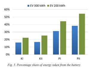
An electric bus equipped with a 300 kWh onboard battery consumes 16% of the energy available during a city cycle. For suburban cycles, the level of energy spent from the battery is 31% for the PI cycle and 38% of the energy stored in the battery pack for the PII cycle.
