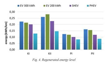
The highest values of recovered energy were obtained for urban cycles. It can be explained by short driving distances and, thus, the need for frequent accelerations and braking. Higher levels of recovered energy were achieved on routes with a varied route profile. Fig. 5 shows the percentage share of energy taken from the electric bus battery after one cycle. The initial battery state of charge (SoC) has been assumed to be 100%.
